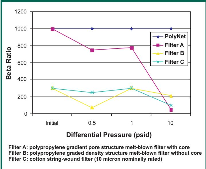
In Figure 1. the following PolyNet PB filters are recommended:
