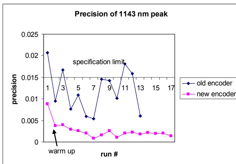
**Figure 1:** Results of Field Acceptance Testing Engineering Study. The precision of the 1143 nm reference peak is plotted for numerous runs before and after the encoder replacement. Note the improved precision of the instrument after encoder replacement.
